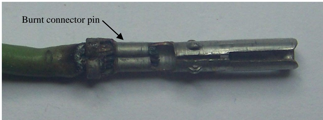
Figure 5. Turn Signal Switch Connector Pin Failure
